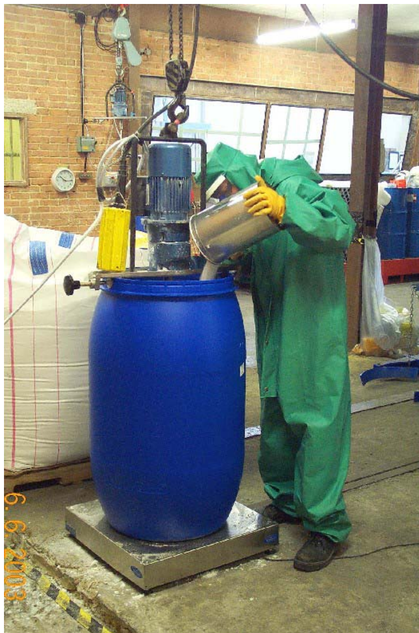
Fig. 4. Adding Granules to HDPE Drum to Solidify Zinc Bromide.
