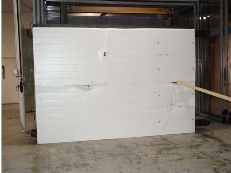
Fig. 8 Complete penetration of wind missile through joint
