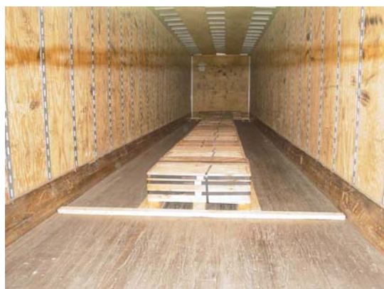
Fig. 4. Trailer loaded with DU metal. Very dense material met truck weight limits long before the volume would be filled.
