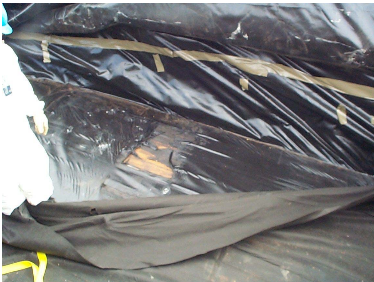
Fig. 3 Damage to the wrapper is shown. The bottom of the rail car shows through the damaged area.
