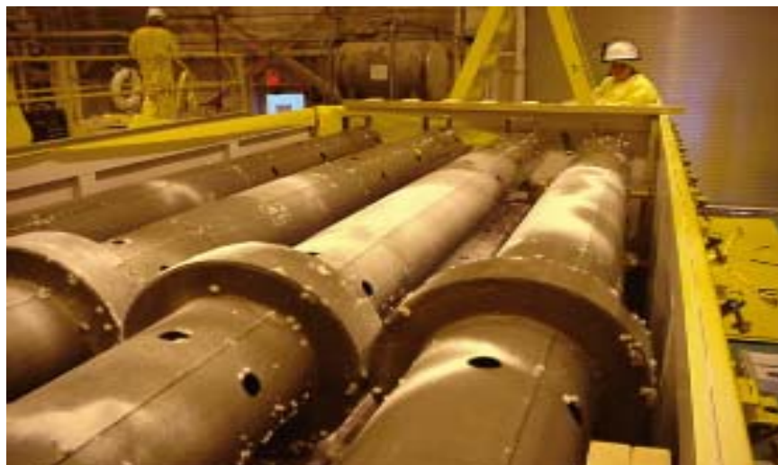
Fig. 2. Canisters prior to foaming (note the flow holes)
