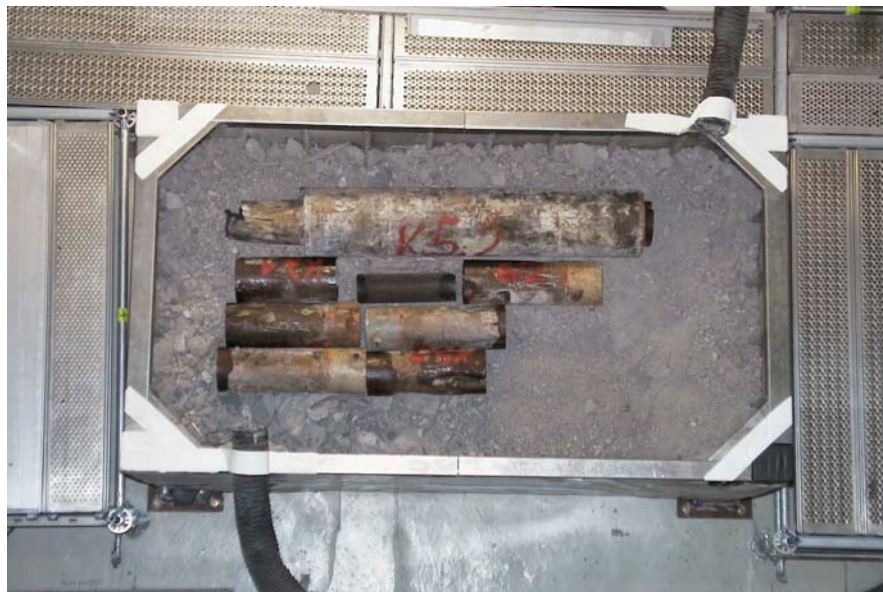
Fig. 3 Waste container with neutron monitor tubes
