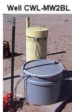
saturated-zone well: water table and sensors ~500 ft below surface
