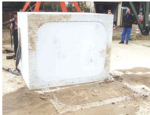
Fig. 4 Box-type Container After 5 m Drop Test onto Simulated Target for Final Storage.
