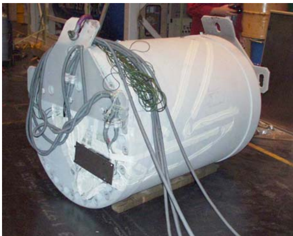
Fig. 3 Prototype MOSAIK ® II Ready for Drop Test at -20^{\circ}\text{C} .
