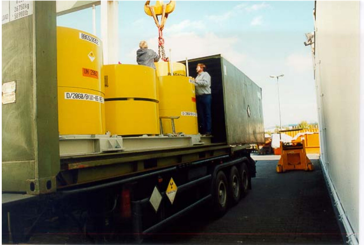
Fig. 3 MOSAIK ® II casks with shock absorbers
