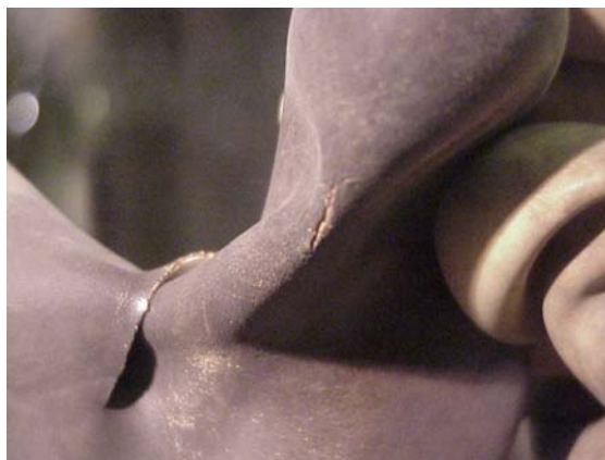
Fig. 2 Example of a crack in a glovebox glove.
