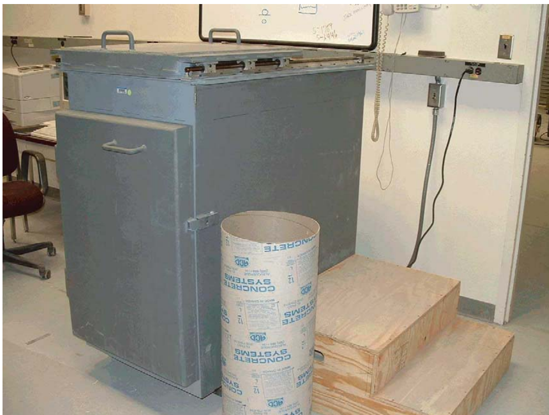
Fig. 1 The ZEUS system detection chamber and measurement cylinder
