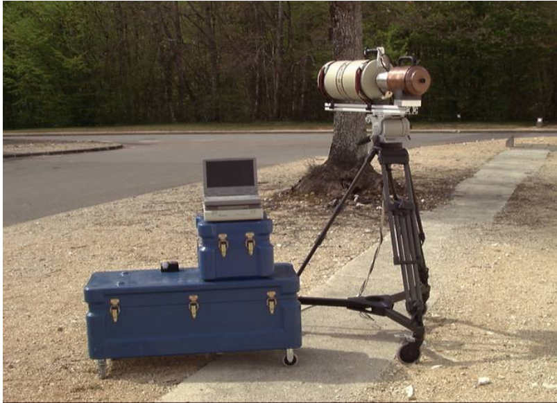
Fig. 2 Mobile gamma detector (HPGe)
