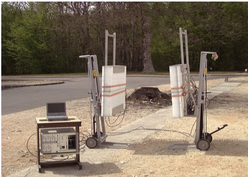
Fig. 3 Mobile passive neutron counter
