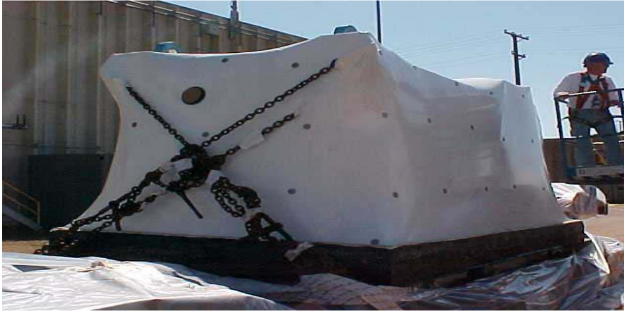
Fig. 5 Shrink-wrapped piece of equipment with thickness measurement buttons
