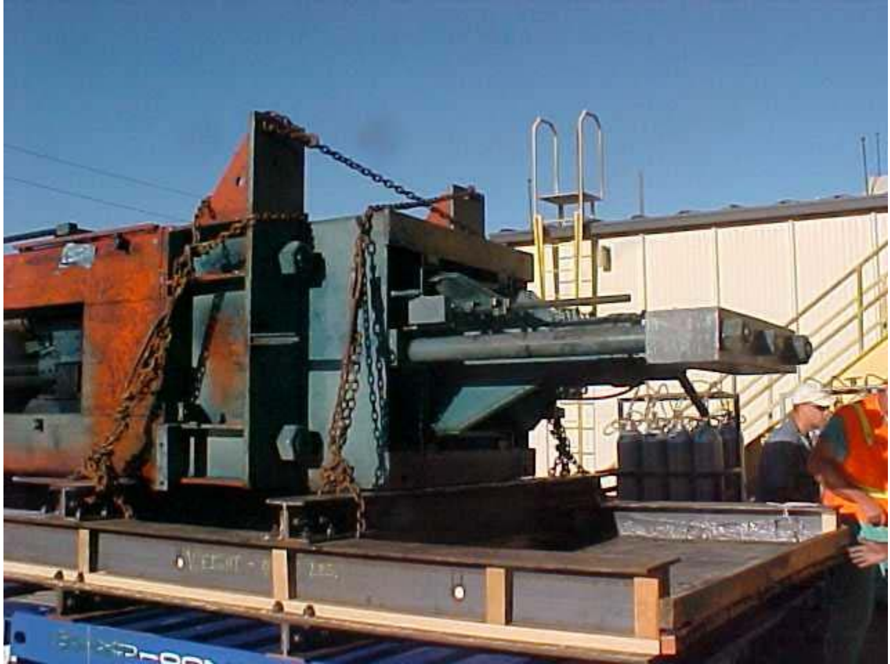
Fig. 4 Extrusion press loaded into prepared base and secured. Ready for shrink wrap.
