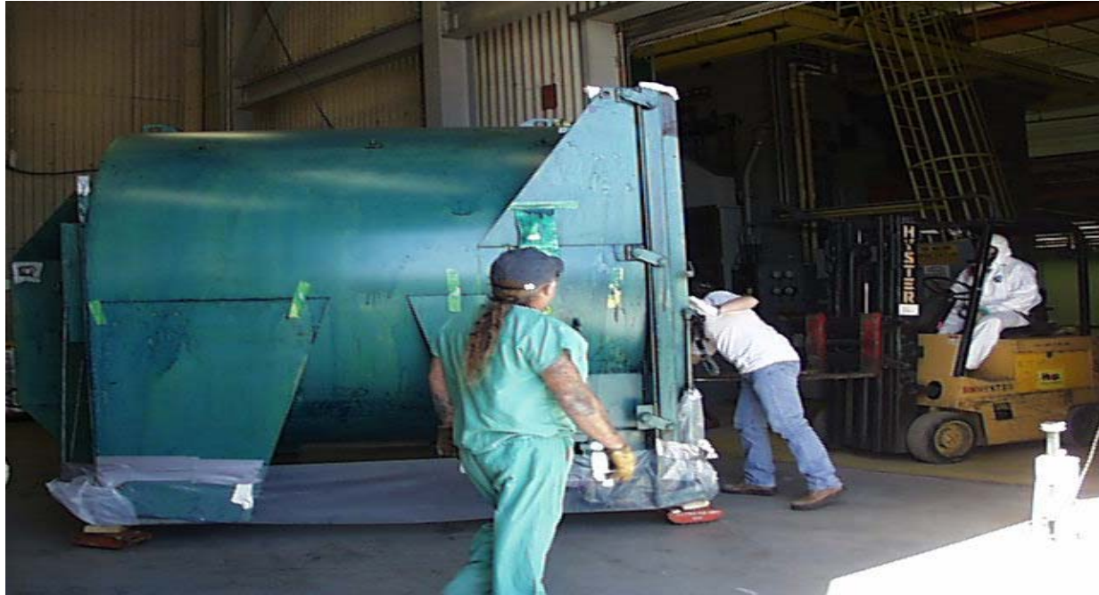
Fig. 1 Oversized be and radiological contaminated production furnace
