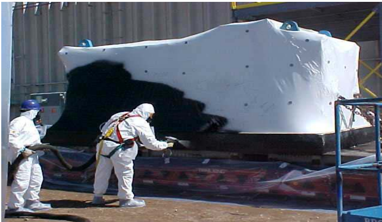
Fig. 6. Spraying InstaCote™ SE on prepared package
