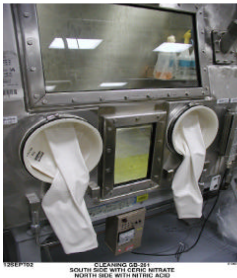
Figure 3. Glovebox used in LANL Cerium (IV) Nitrate demonstration
