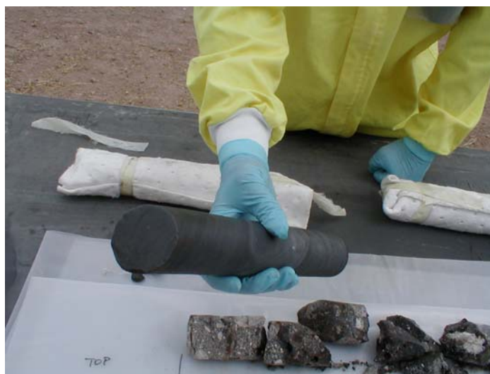
Fig. 2. Glass core from the NTISV hot test demonstration at MDA V. Note transitional tuff/glass material collected from the top of the melt (approximately 3 m [10 ft] bgs) on the table.
