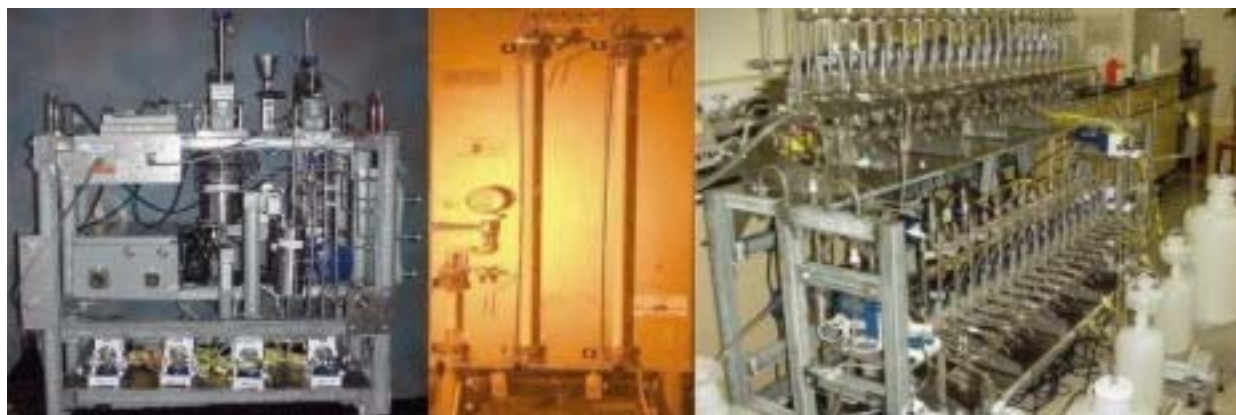
Fig. 1. Main processing equipment for the demonstrations, from left to right: precipitation, ion exchange, and solvent extraction.
