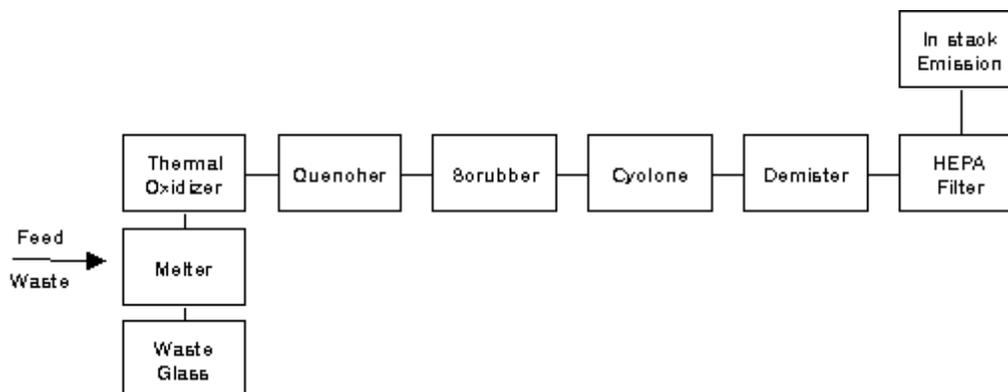
Fig. 1 Flow diagram of pilot-scale vitrification plant PAM
