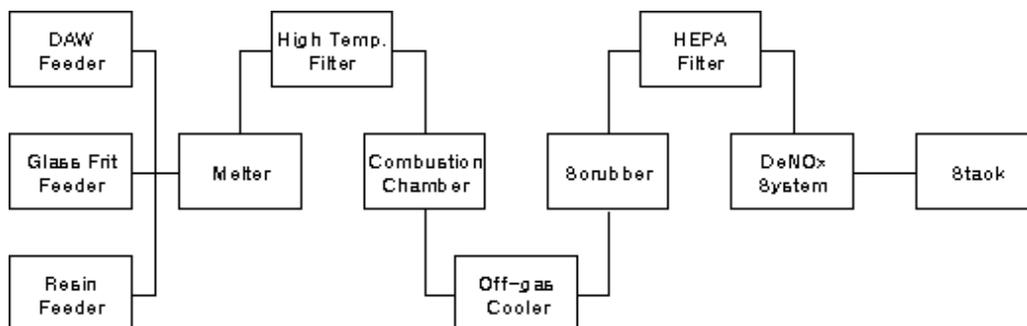
Fig. 2 Flow diagram of pilot-scale vitrification plant CCM
