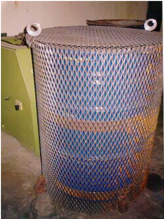
Fig. 3 Sample of degraded package inside the basket
