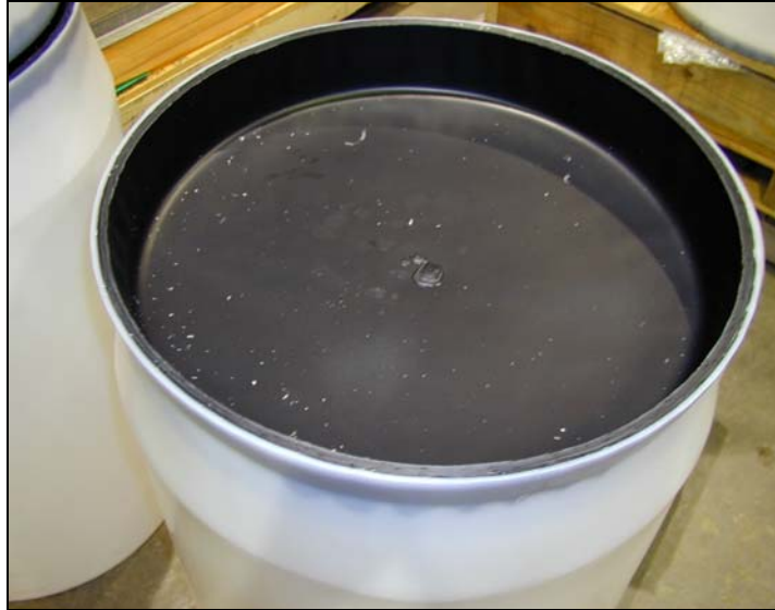
Fig. 3. Successfully welded liner.
