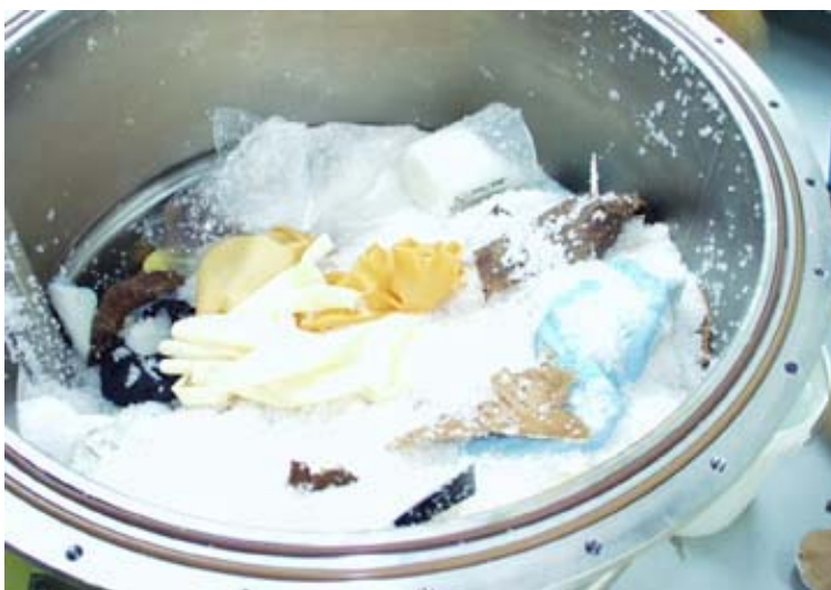
Fig. 3 Absorbed Brine and Mock Waste Materials
