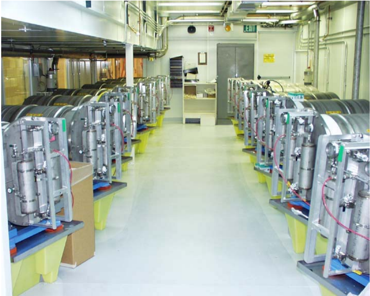
Fig. 1 250-liter Containers With WIPP-type Brine and Waste
