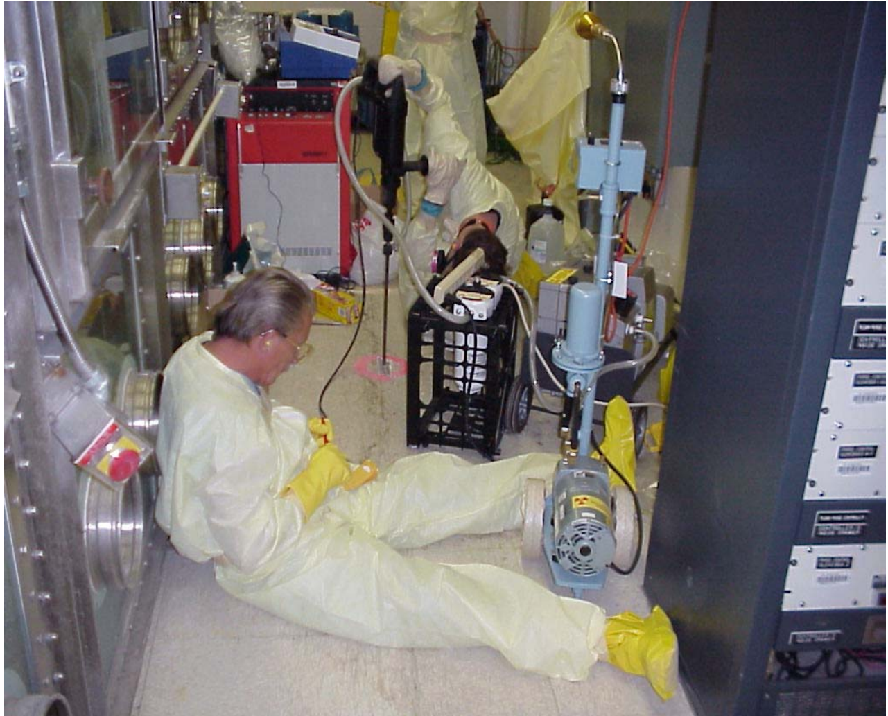
Fig.1. Use of RadPro™ To Sample & Characterize Concrete Floors of Nuclear Facilities
