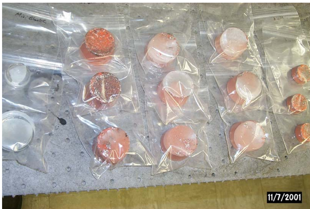
Fig. 4. Typical "Hockey Puck" samples prepared as mock-ups for leaching tests
