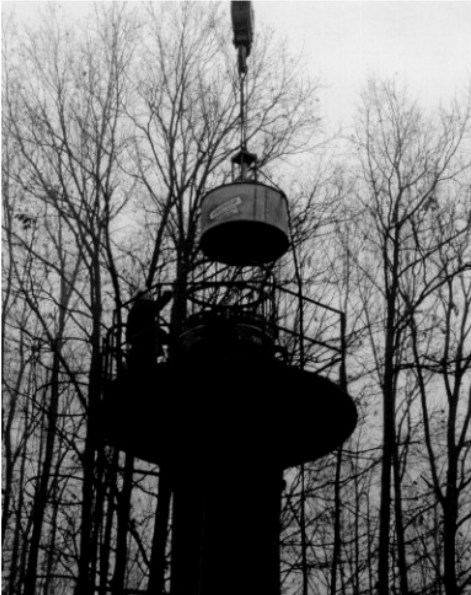
Fig. 3. The basket during preparing of the 7m drop tests
