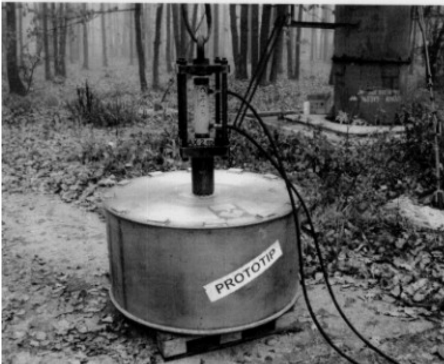
Fig. 1. The prototype of the CANDU spent fuel storage basket
