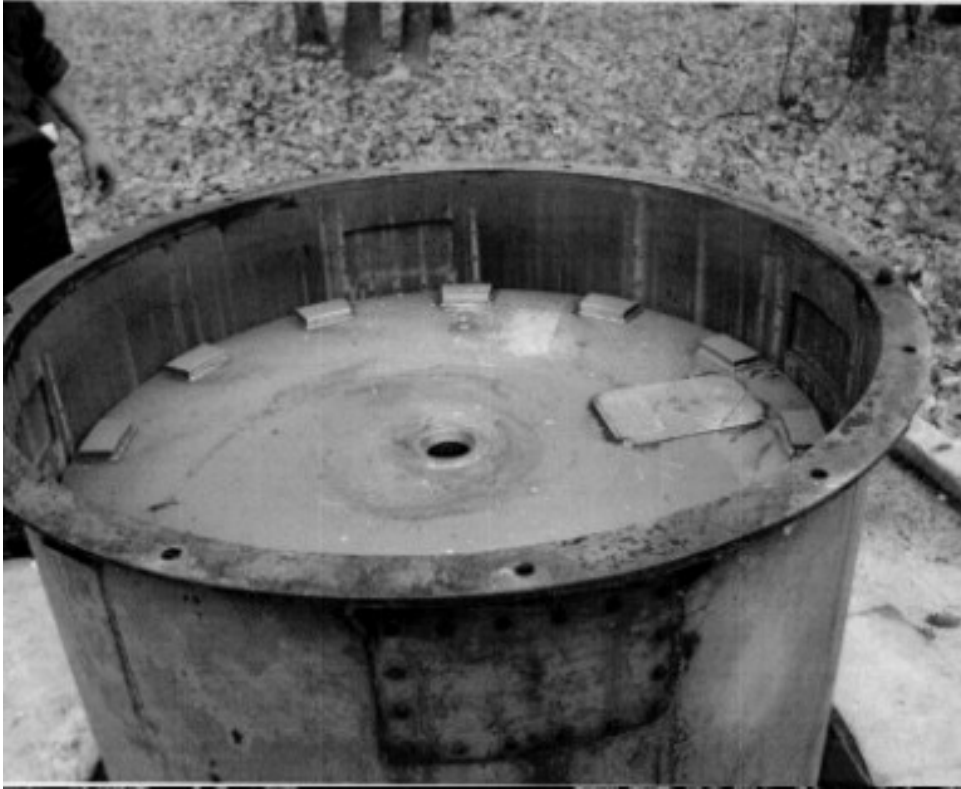
Fig. 4. The CANDU spent fuel storage basket prototype after the 7m drop tests
