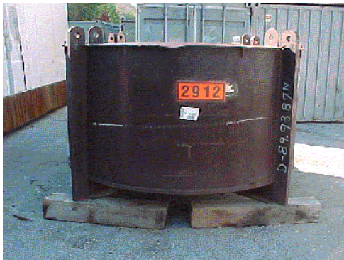
Fig. 3. Lead-lined cask with accelerator beam magnets
