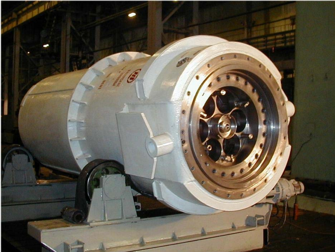
Fig. 2. AMEC TUK-108 prototype cask without lids and one fuel canister installed.
