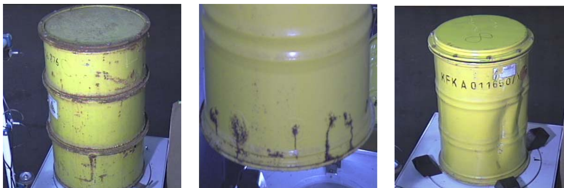
Fig. 3: Examples of corroded or damaged drums
