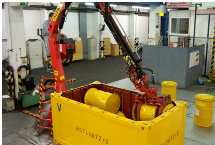
Fig. 4: Packing of 14 200-l-drums per steel container
