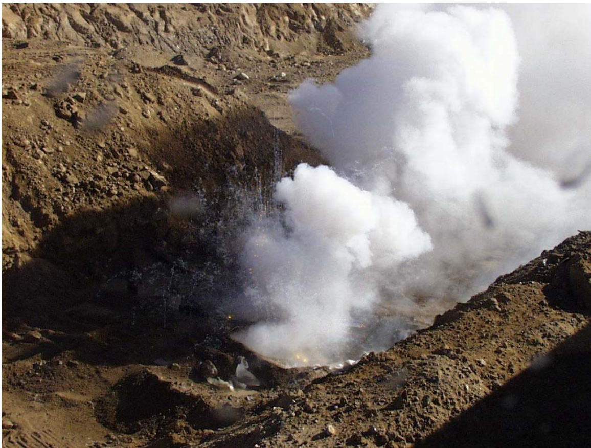
Fig. 3. Reaction of sodium-potassium compound with water
