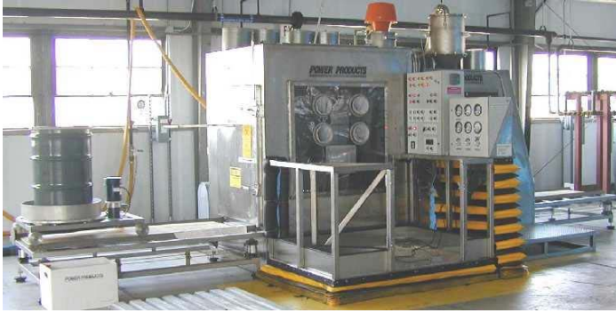
Fig. 2. Drum Repackaging Station, Unit 1 (two views)
