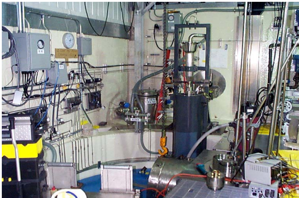
Fig. 5. UDR charcoal removal equipment at ACB
