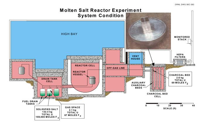
Fig. 3. Diagram of MSRE design<sup>b</sup>, with an inset photographic enlargement of lead-cap shield.
