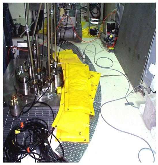
Fig. 4. Lead Blankets over the Source.
