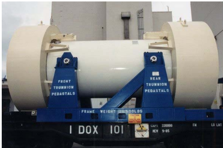
Fig. 4 - WVDP fuel was loaded into two shipping casks like this one for future transport to INEEL in Idaho
