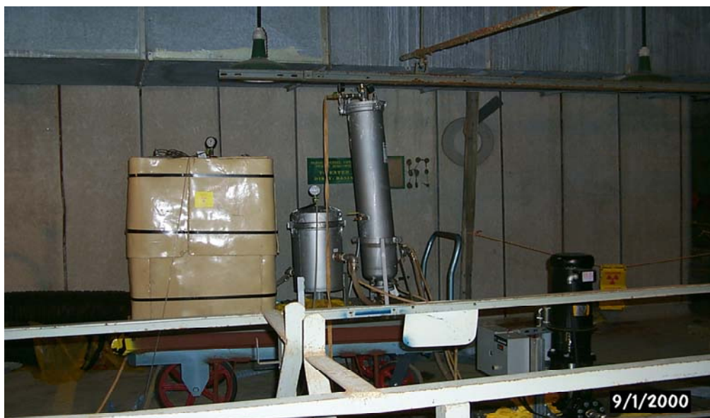
Fig. 2 – 3M Cs-137 Removal System in the R-Reactor Disassembly Basin. The 4-foot tall, 6-inch diameter, 2-micron pre-filter is to the right and a small tank with nine 0.2-micron pre-filters is in the center. The 22 SSC™ Cs-137 removal filters are inside a stainless steel tank to the left, which was covered with ~1 inch of lead shielding to reduce the gamma dose.
