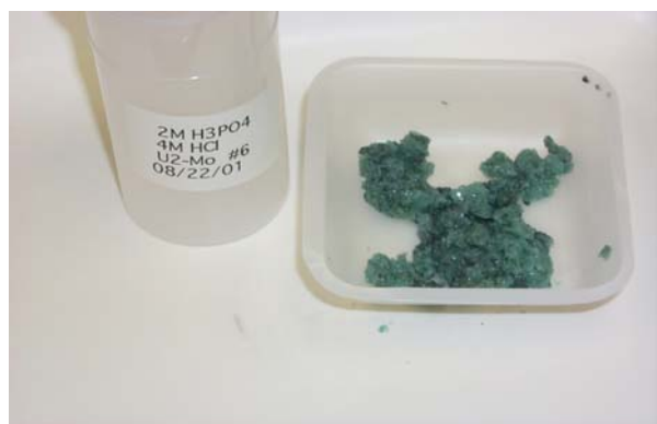
Fig. 5. The solid from test tube in Fig.4 was removed from the tube. No free liquid was noted.
