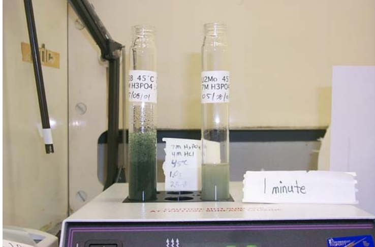
Fig. 2. Dissolution of one gram of both types of Dep-U studied with 7M H_3PO_4 is complete within 1 min at 45°C.
