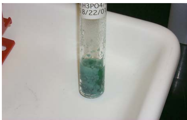
Fig. 4. Tube containing uranium precipitate formed following dissolution with \text{H}_3\text{PO}_4/\text{HCl} . (10 mL/1 g, T= 25, dissolution time = 15 min)
