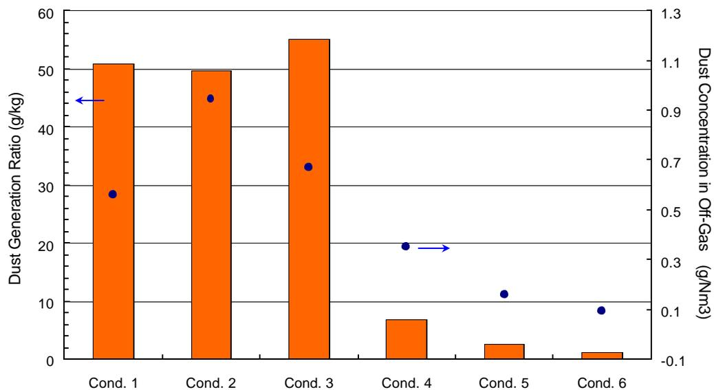
Fig. 2. Dust generation ratios (bar) and average dust concentrations (●) in off-gas on the operating conditions for PE waste vitrification
