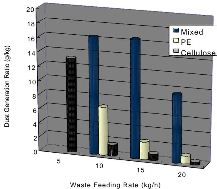
Fig. 3. Dust generation ratios for three waste types on the waste feeding rates
