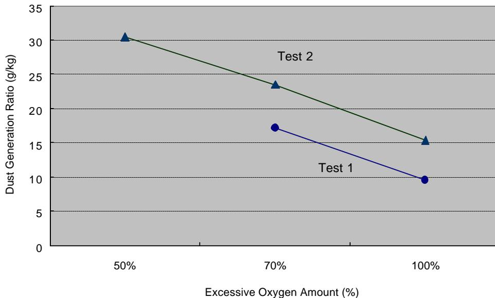
Fig. 4. Dust generation ratios on the excessive oxygen amounts for the mixed DAW vitrification tests
