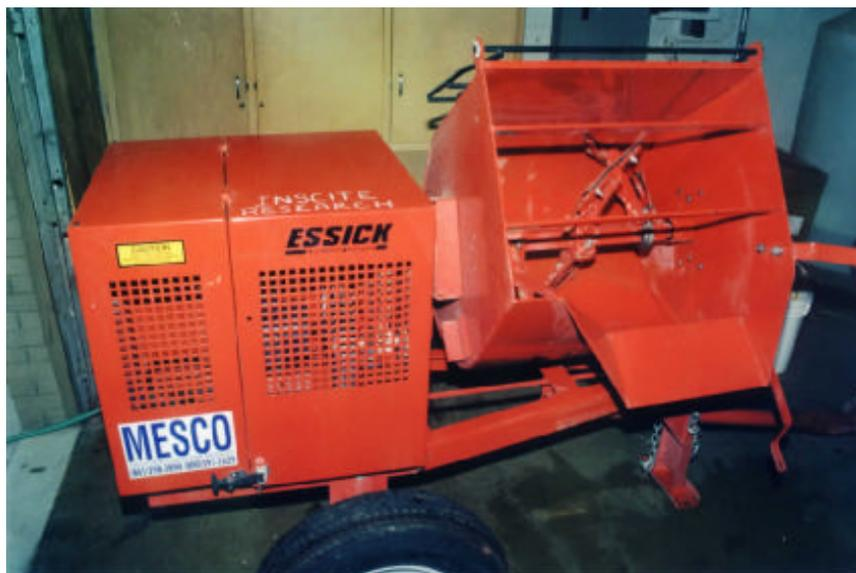
Fig. 1. Commercial Mortar Mixer Used for Demonstrations
