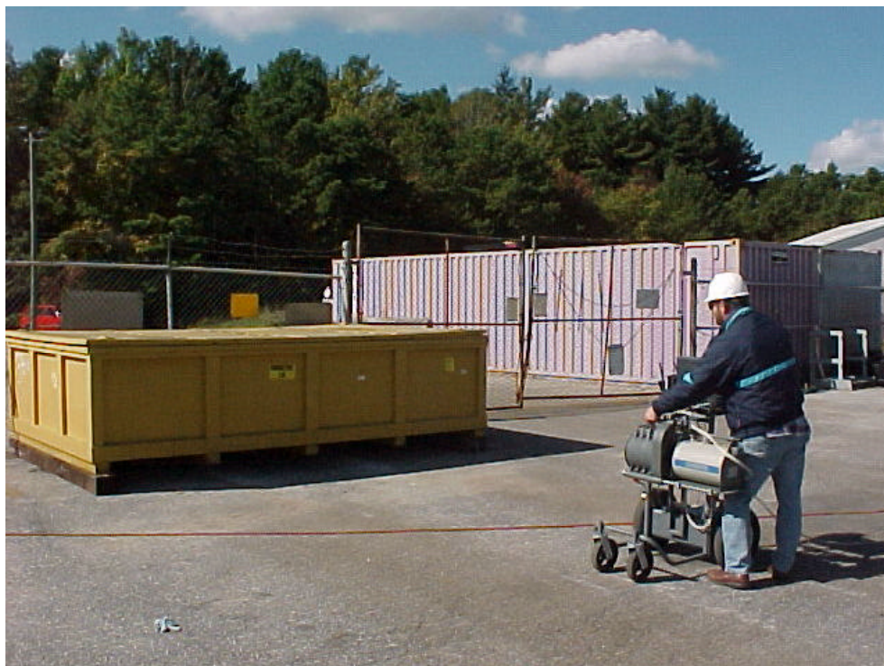
Fig. 1. Spectrum Acquisition on B-25 Waste Container
