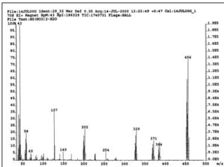
Fig. 2. DIP mass spectrum of mercuric nitrate monohydrate
