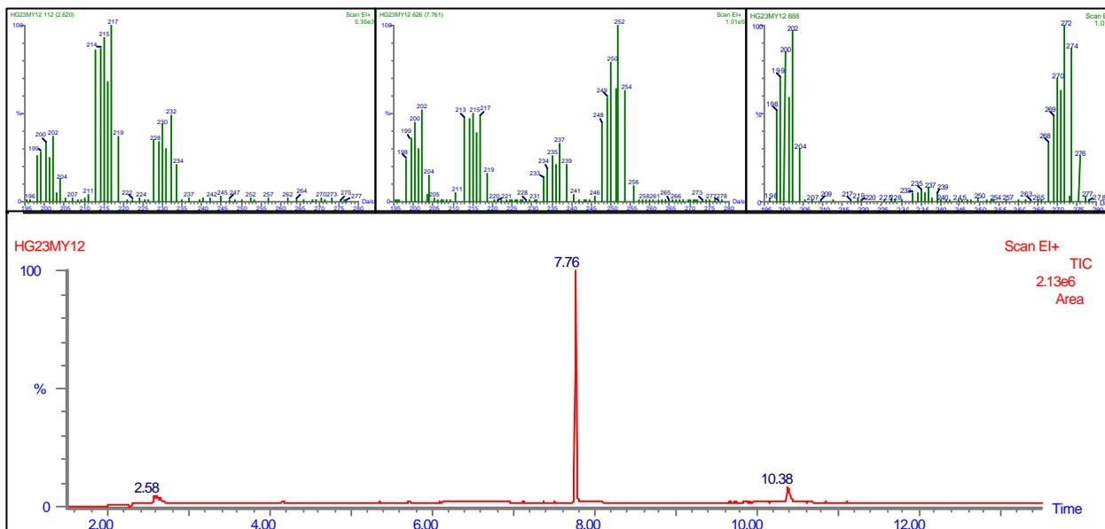
Fig. 4. Chromatogram and correspondent mass-spectrograms of dimethylmercury, methylmercury chloride, and mercuric chloride mixture
