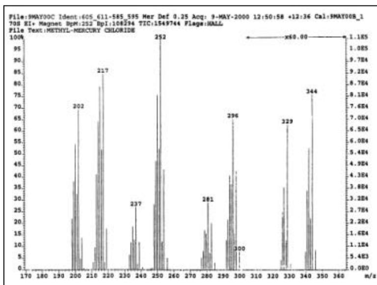
Fig. 3. Direct probe mass spectrum of methylmercury chloride
