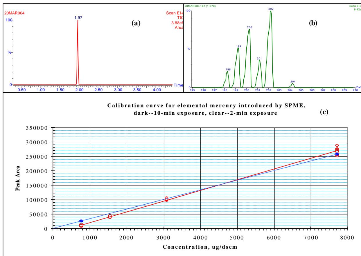
Fig. 1. a) Elemental mercury chromatogram; b) SPME sampling (CAR/PDMS, 75 μm, phase, black), 60-sec exposure, column ZB-WAX, isothermal run at 25 °C; a corresponding mass spectrum; and c) calibration curves
