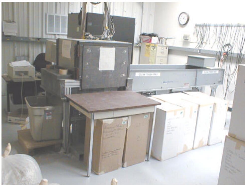
Fig. 1. The WAND System. Detectors are housed to the left of the conveyor belt.
