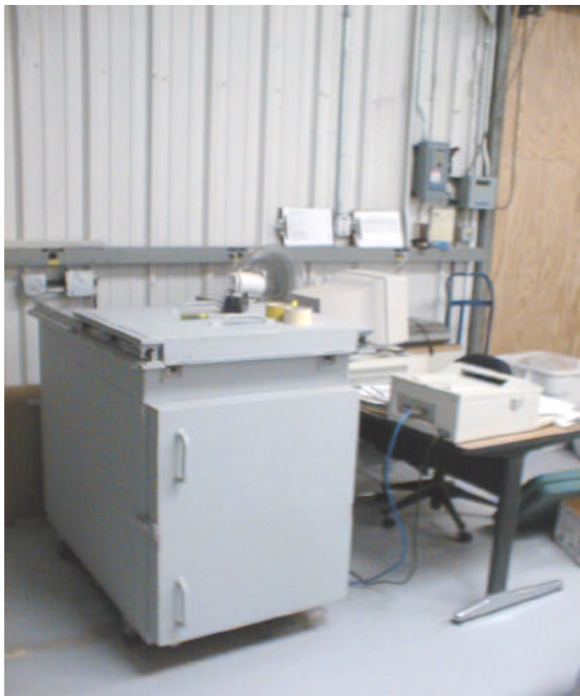
Fig. 2. The HERCULES System. Detectors are housed on the near side of the chamber, waste is placed on the far side.
