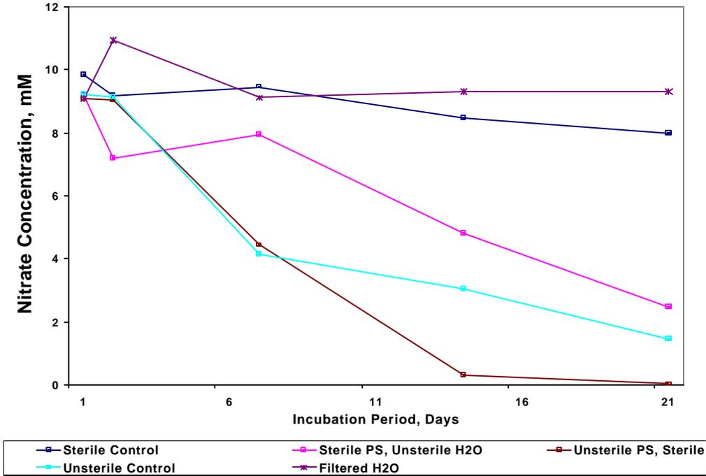
Fig. 1. Biodegradation of nitrate in Mortandad Canyon groundwater supplemented with 9.7 mM nitrate using a pecan shell biobarrier support material.
