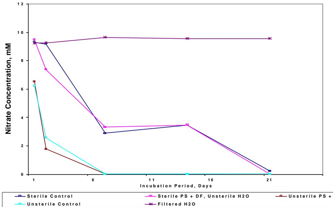
Fig. 2. Biodegradation of nitrate in Mortandad Canyon groundwater supplemented with 9.7 mM nitrate using a pecan shell and dog food biobarrier material.
