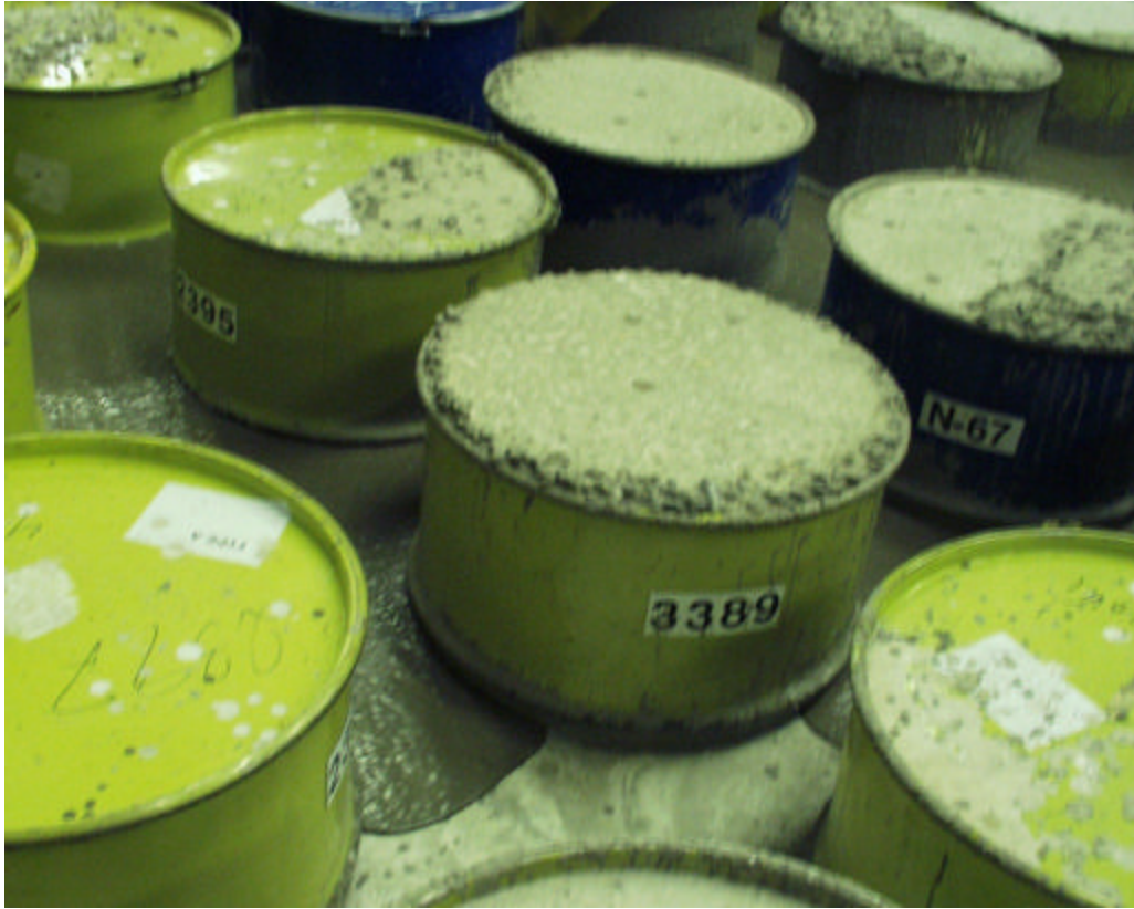
Fig. 3. Encasing of drums in cement. The first layer (to mid-drum) is poured.
