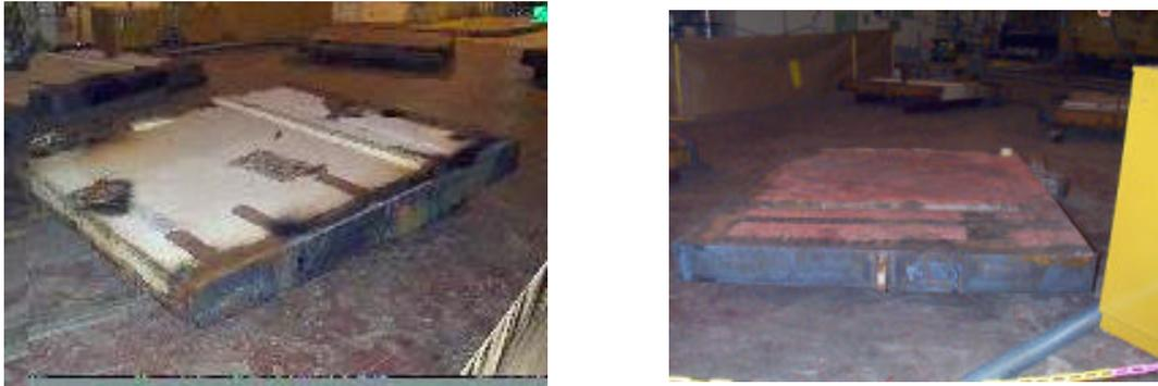
Fig. 5. Before and After Paint Removal Process
