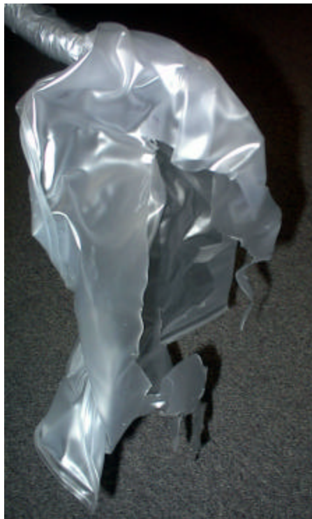
Fig. 3. PVC Bag breached using UltraTech's Inner Layer of Confinement Reduction Method
