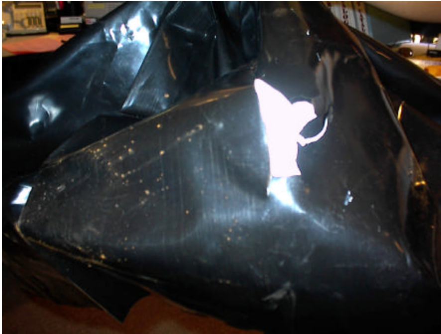
Fig. 4. Eight mil polyethylene 55-gallon liner after the LN2 injection and evacuation process
