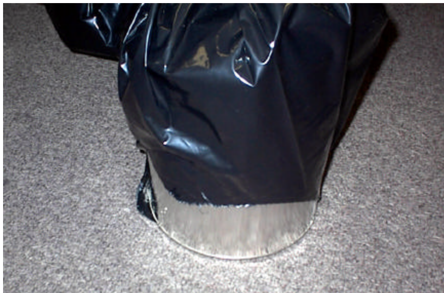
Fig. 5. Breached polyethylene bag that was tightly sealed around a paint can filled with sand
