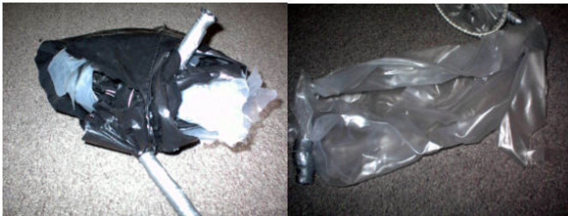
Fig. 2. Six layers of polyethylene bags breached (on left) and one layer of a PVC bag breached (on right)
