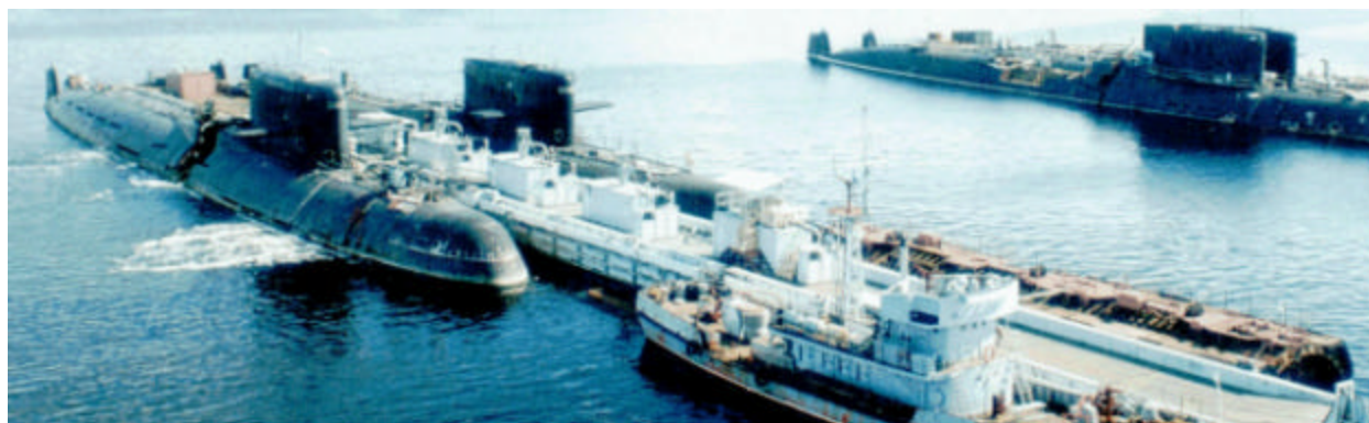
Fig. 1. The ETPP injecting polystyrene into decommissioned submarines.
