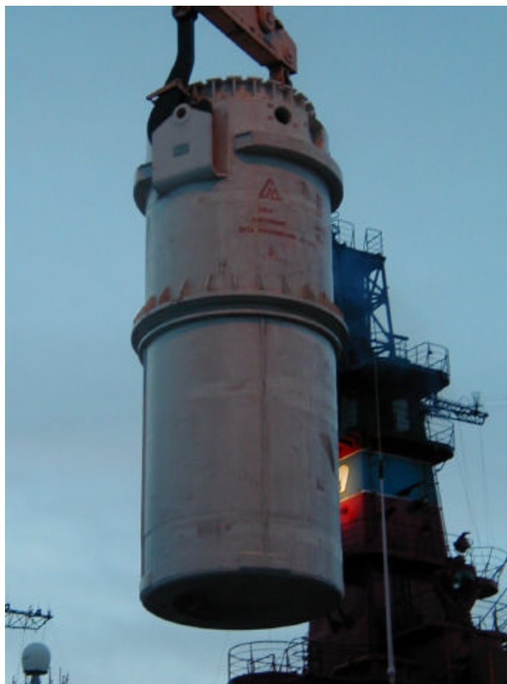
Fig. 2. AMEC cask undergoing testing at the RF RTP “Atomflot” site.
