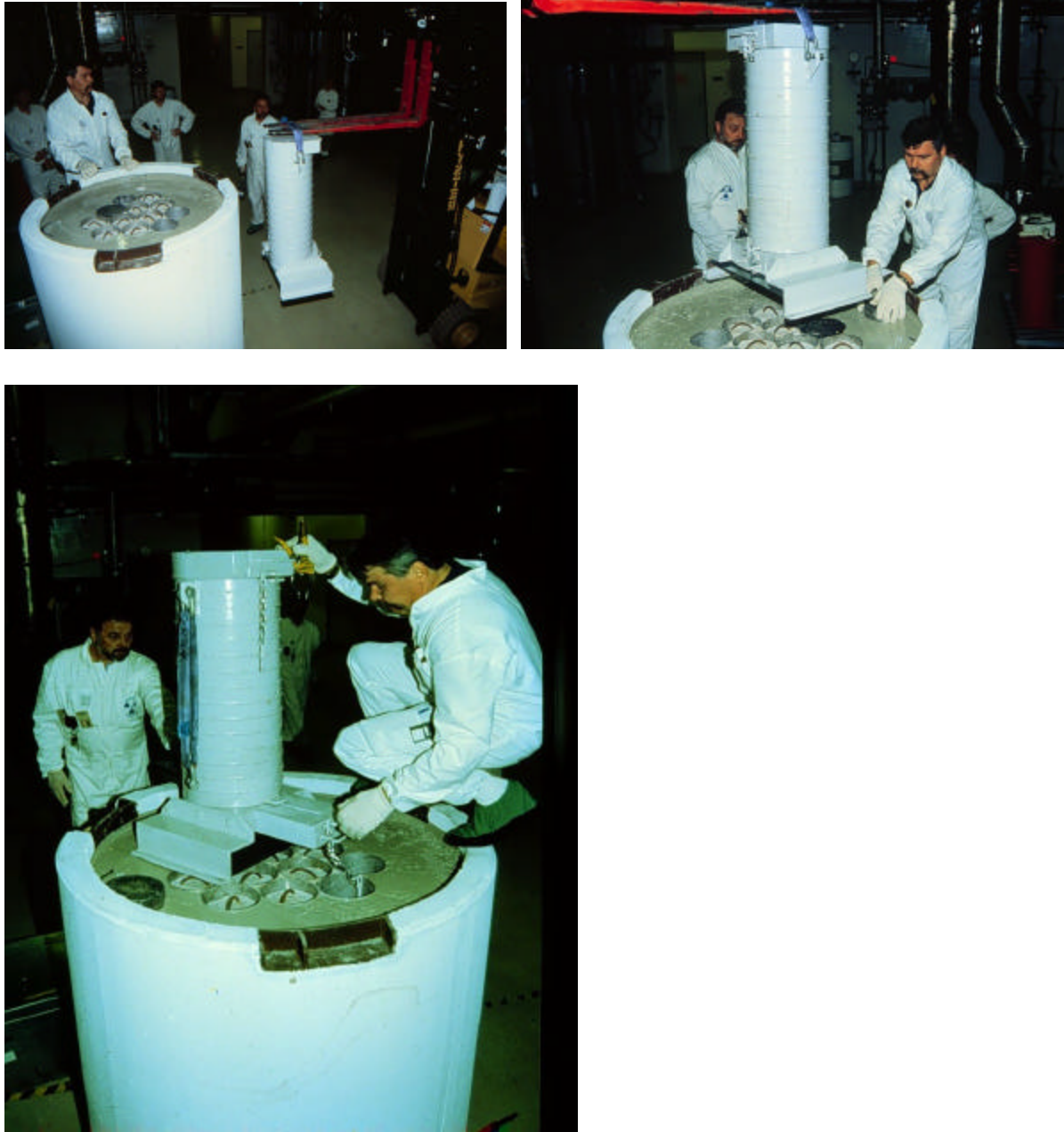
Fig. 1. Used ion exchange columns are disposed of in concrete containers. One container can have cesium from about 1000 m 3 of high-salt evaporator concentrate.
