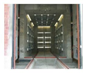
The UWM shown in Figure 3 is a unique passive neutron counter (PNC) capable of accurate uranium assay for a range of freight containers including Intermodals, ISO (SeaLand) containers, ST90 boxes, and drum packs. To achieve this the system employs 80 polyethylene clad neutron counting modules [known as DISPIM®] together with electronics that provides regulated high voltage distribution, signal conditioning and amplification for 12 independent neutron counting
