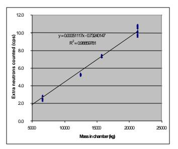
Fig. 6. Spallation effect on Carbon Steel
