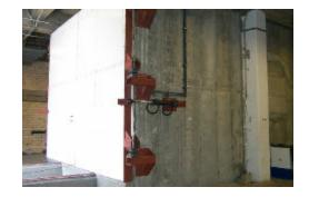
Fig. 4. Shielded Chamber Door
