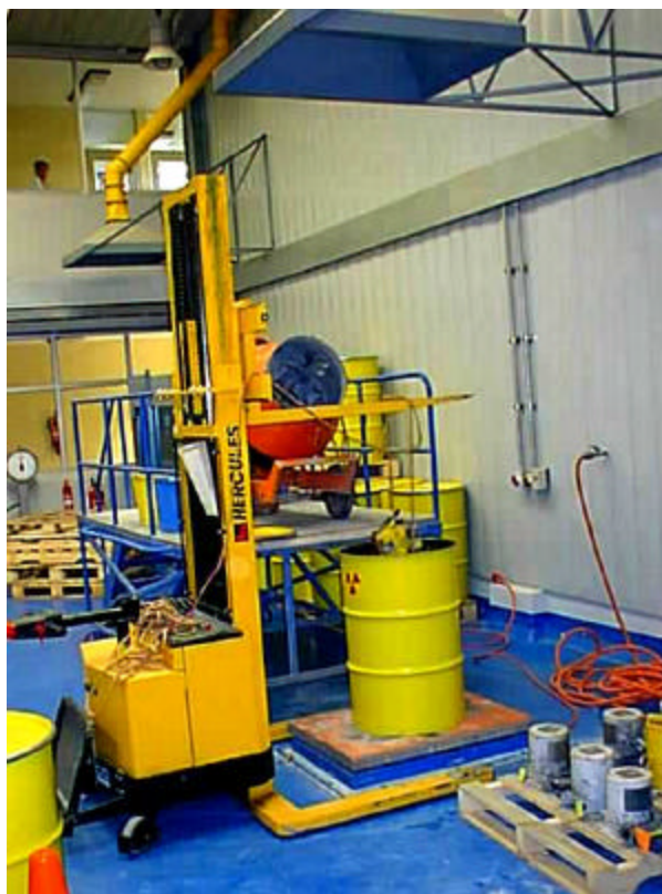
Fig. 1. Direct conditioning of spent sealed sources
