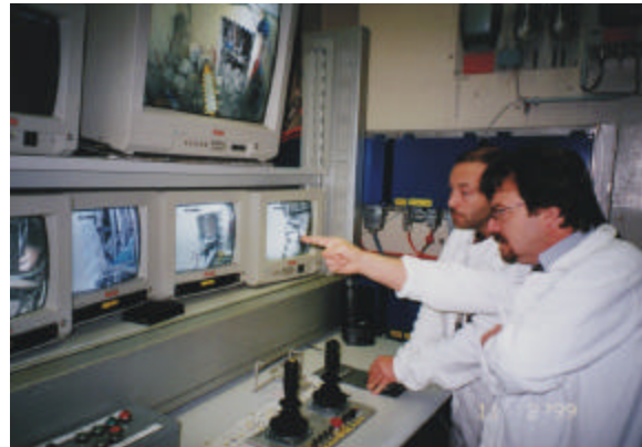
Fig. 1. Horizontal remote dismantling equipment (crawler digger Brokk 150) and control panel
