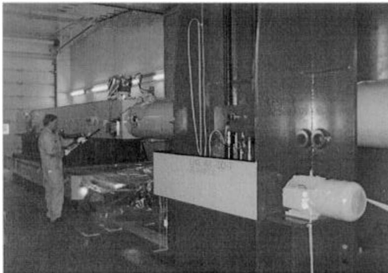
Fig. 5. Transfer of the transport cartridge from the shielding tube of the tilting device into the shielding container (level+0m)
