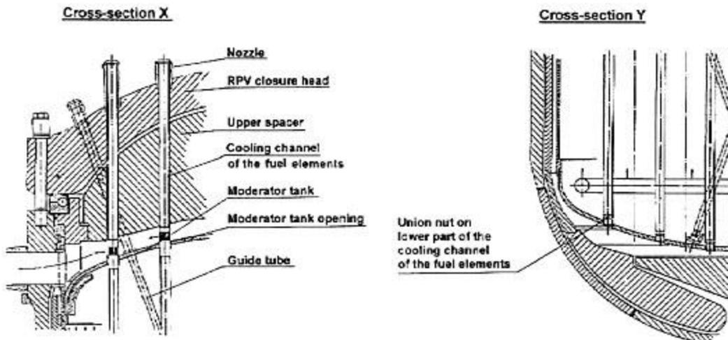
Fig. 3b. Rod-shaped components above and inside the RPV: Cross-sections X and Y
