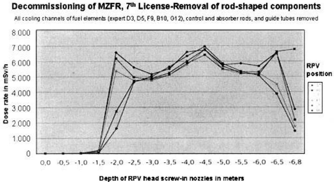
Fig. 6. Dose rate as a function of depth of measurement and position
