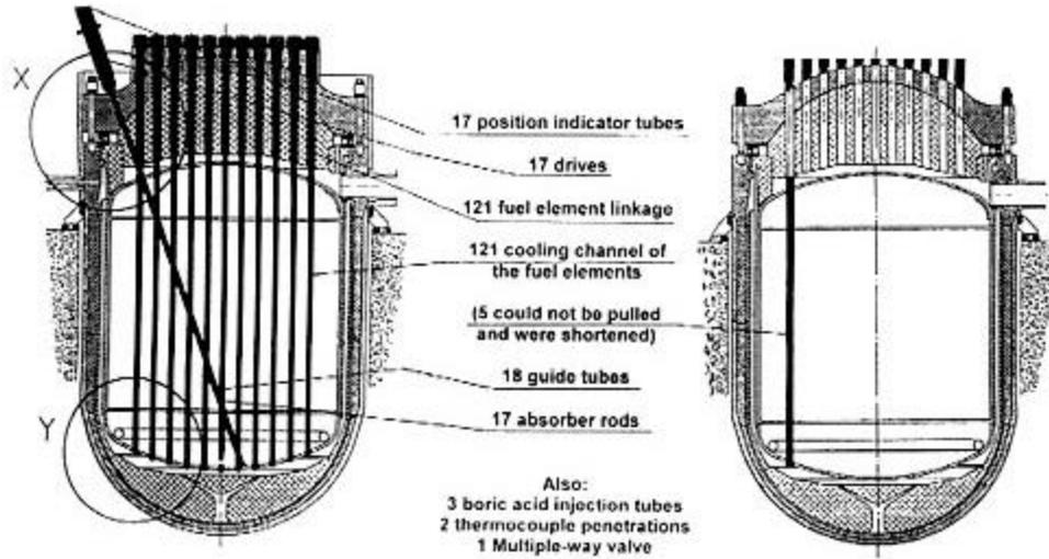
Fig. 3a. Rod-shaped components above and inside the RPV before removal of rod-shaped components (left) and after removal of them (right)
