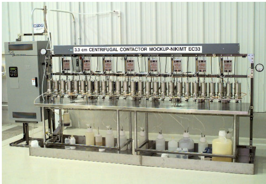
Figure 2. 3.3-cm centrifugal contactor pilot plant
