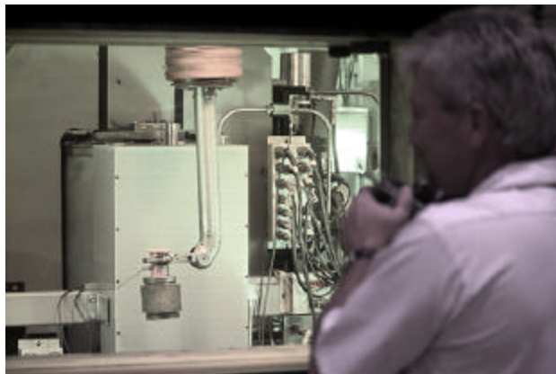
Fig. 2. Hot Isostatic Press in the Hot Fuel Examination Facility (background) and the First Irradiated Ceramic Waste Form Product (held by manipulator)
